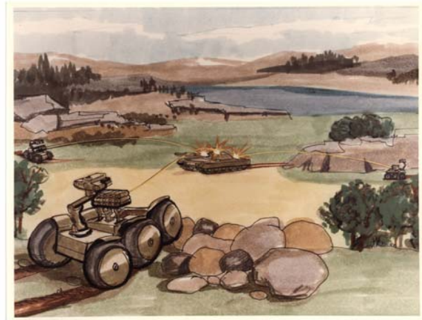
Figure 17: 1985 TARDEC Concept Articulated UGV engaging enemy armor with anti-tank weapon
