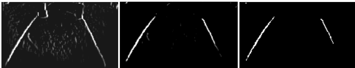
Fig.14(a): Image after the Sobel mask applied to the blue plane. (b): Sobel.*blue. (c):After threshold.
